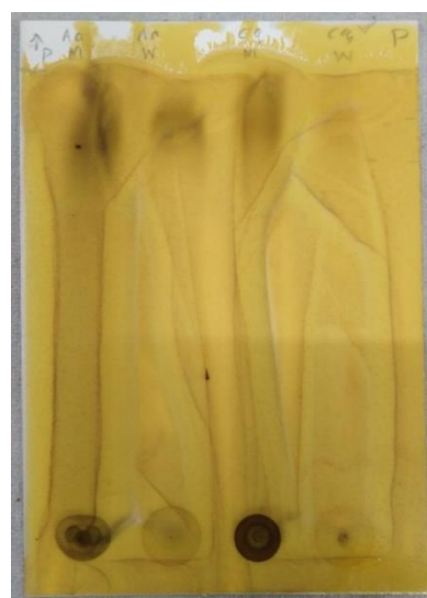
Figure 9: TLC separation of phenolic compounds: after derivatization with confirmatory spray agent 10% ferric chloride.
