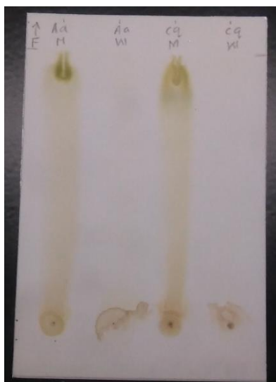
Figure 5: TLC separation of flavonoids: before derivatization.
