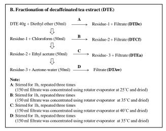
Figure 1: Detail process of extraction and fractionation
